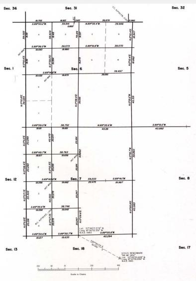
This plat represents the retracement of portions of the west and north boundaries and the subdivision lines; and, a corrective resurvey of a portion of the subdivisional lines and the subdivision of sections 6 and 7, T. 35 S., R. 3 E., Salt Loke Merdian, Utah, superseding that portion of the survey executed by Gail E. Reynolds Supervisory Cadastral Surveyor, in 1980–83, Group No. 603, Utah.
